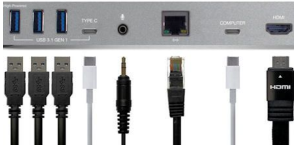
Figure 2. OWC's USB-C dock gives ultralight computers desktop-PC I/O capabilities.
